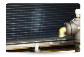
All models in the TREF DX range feature heat exchange coils with hydrophilic coating. This special coating, together with an adequate adjustment of air through flow speeds, helps condensate collection during the dehumidification process, avoiding dripping on the inside and outside of the unit.
